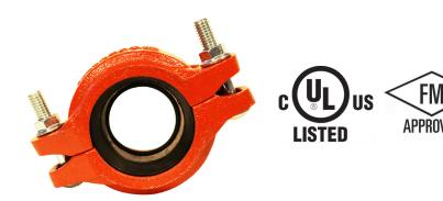
The ARGCO Model 105 reducing coupling allows for direct reduction on a piping run and eliminates the need for a concentric reducer and couplings. The specially designed rubber gasket helps prevent small pipe from telescoping into larger pipe during vertical assembly.
